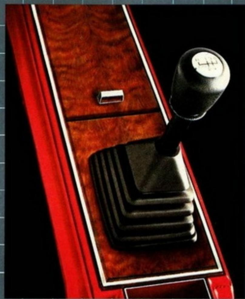
*Five-speed manual transaxle.* A real driver's option, synchronized in all forward gears, with an integrated overdrive fourth gear. (Not available on two- and four-door base models.)
