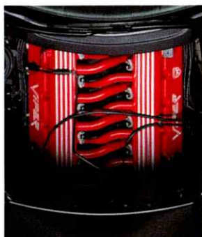
Viper's aluminum V10 engine.
