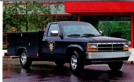
The midsize Dakota Chassis Cab can carry up to 2,800 pounds of payload with the standard Magnum 3.9-liter V6 engine. This one is shown with a galvanized steel service body.
