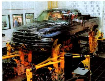
Laboratory isolation testing on the suspension "Shaker" (Road Test Simulator) uses computer re-creations of the nation's roughest roads to punish vehicles far longer and more severely than any real-world driver could endure. Testing 18 days on the Shaker equals a 16-week, 20,000-mile endurance run.
