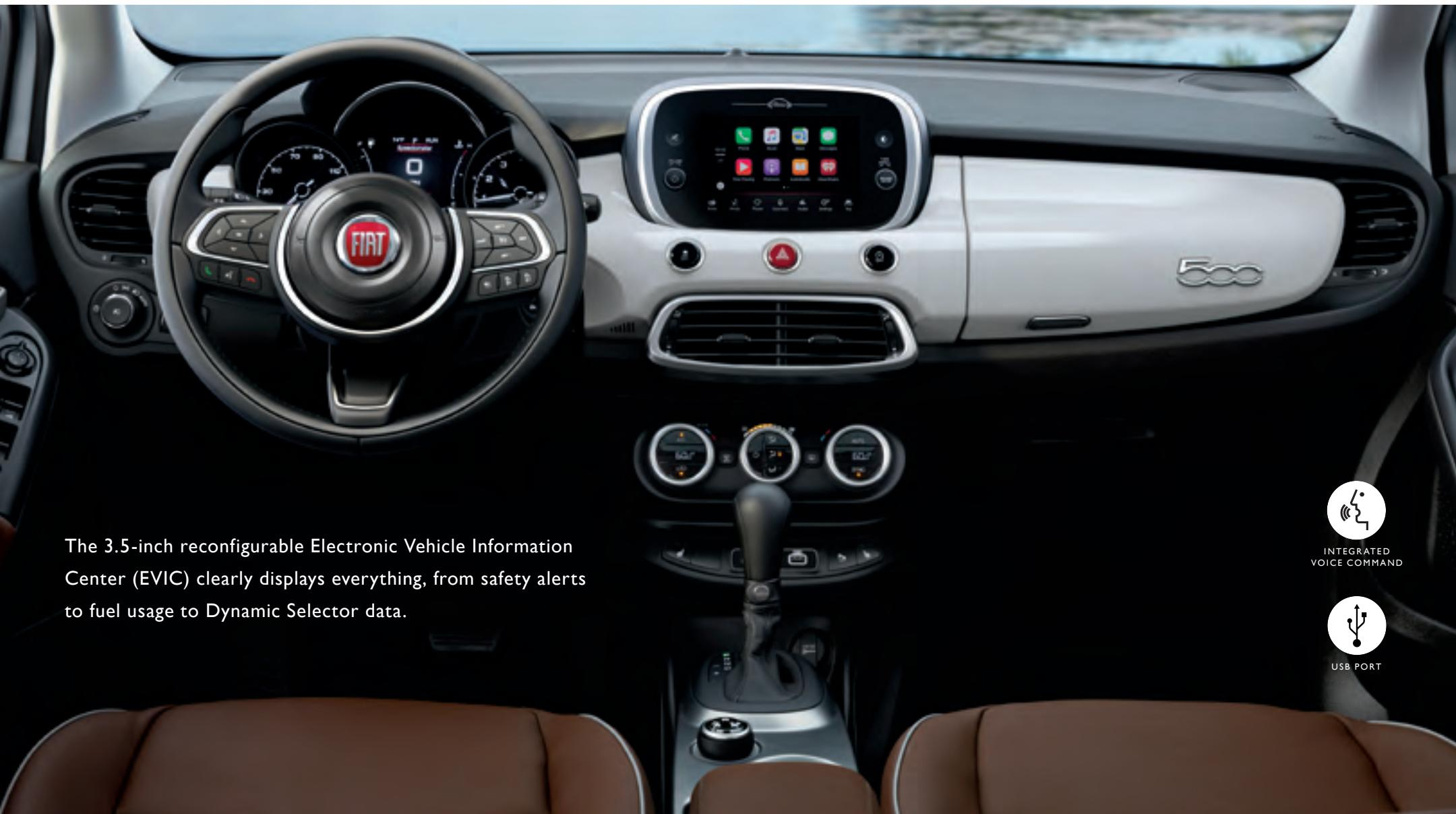
The 3.5-inch reconfigurable Electronic Vehicle Information Center (EVIC) clearly displays everything, from safety alerts to fuel usage to Dynamic Selector data.
