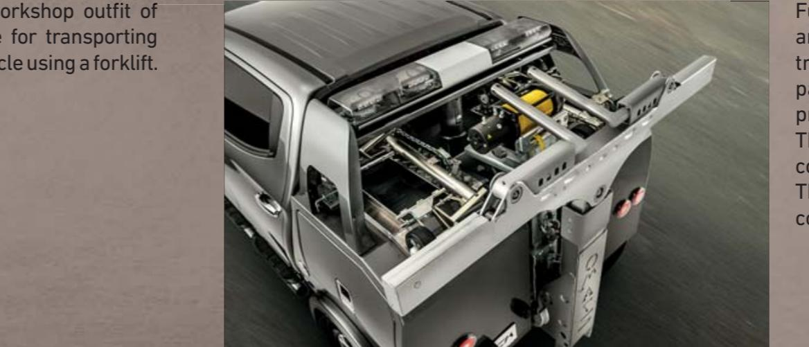
Specific roadside rescue workshop outfit of the rear part of the vehicle for transporting equipment and towing a vehicle using a forklift.
