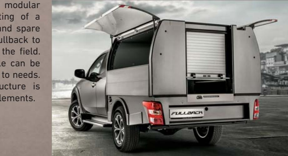
Fullback Mobile Workshop is a modular and reconfigurable outfit consisting of a transport system for equipment and spare parts fitted onto the chassis of Fullback to provide maintenance services on the field. The three elements of the module can be combined and equipped according to needs. The aluminium section bar structure is complete with synthetic material elements.
