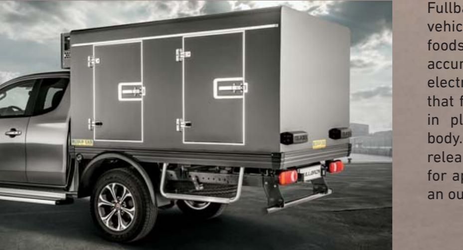
Fullback Refrigerated Body is the ideal vehicle for daily distribution of frozen foods at cold temperature. The cold is accumulated while parking at night by an electrically operating refrigeration unit that freezes an eutectic solution contained in plates or tubes arranged inside the body. By defrosting the eutectic solution releases the previously accumulated cold for approximately 10 hours of service with an outside temperature of +30°C.
