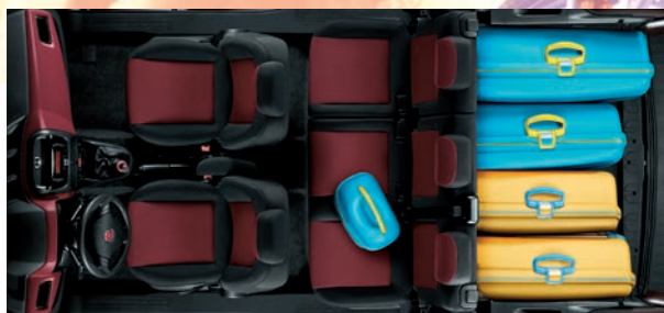
Long and flat load platform with folded passenger seat and parcel shelf at lower level.
