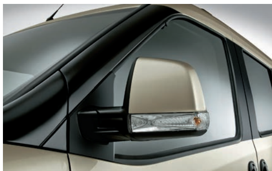
Door mirrors with built-in direction indicators.
