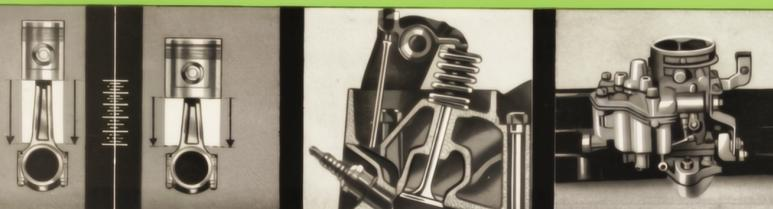
**OVERSQUARE, SHORT-STROKE DESIGN:** The most efficient power in modern engines comes from oversquare design in which the diameter of the cylinders is increased in relation to their depth. This allows a shorter piston stroke which lessens internal friction, saves wear and gets more efficiency from less petrol. On the right, above, is illustrated Consul's "short-stroke" of piston in comparison with that of the conventional engine as shown on the left.
