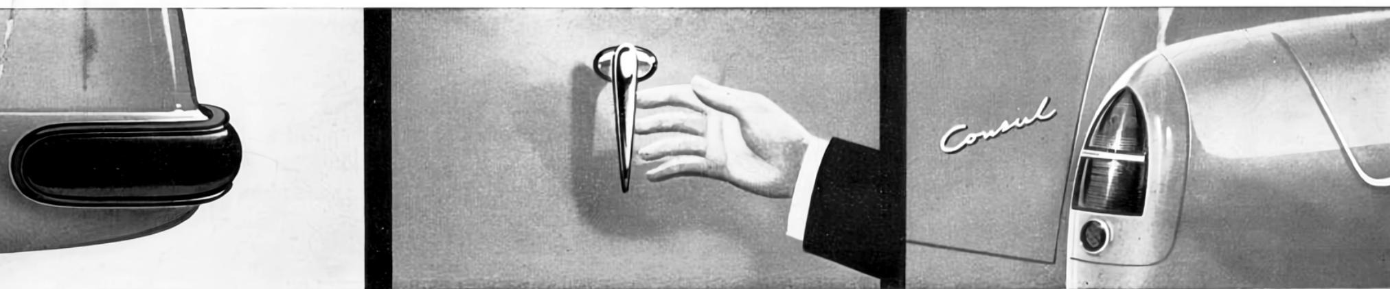
**REAR END PROTECTION.** Rubber-faced bumperettes curve right around the vital rear corners, absorb shocks better and do not show scratches.
