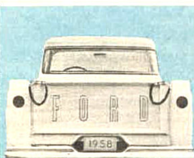
The rigid construction of the box-like corner posts—with the steel tailgate and toggle-type latches—gives you unequalled body strength and rigidity.
