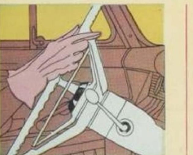
**Safety steering wheel.**—The dish type form of the steering wheel permits the use of a shorter steering column, the upper end of which is therefore farther away from the driver's body—and furthermore the steering wheel is made of flexible material.
