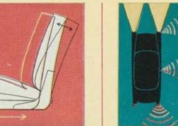
**Front seats adjustable in two ways.**—Not only the front seat is adjustable but also the position of its back rests may be changed individually and independently of the bench. This combined seat adjustment makes it possible to arrange seats in such a way as it is most comfortable for driver and passenger.
