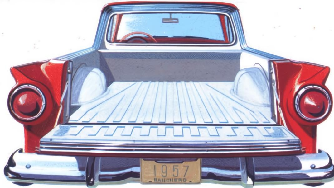
**Hauls like a truck!** How big do your loads come? The Ranchero takes 'em all the way up to 1,190 pounds! Body is full size, with double flooring for extra strength and rigidity. Closed, the tailgate is locked by an external handle. Lowered, it extends the level floor length to nearly eight feet.
