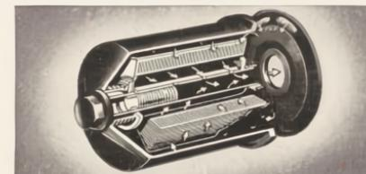
**Full Flow Oil Filter** cleans ALL the engine oil before it reaches bearing surfaces, reducing cylinder wall and piston ring wear and thereby contributing to longer bearing life.
