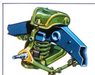
Ford's 4-Way Ball-Joint front suspension has one-piece lower and upper suspension arms. Lower arms are swept back so front wheels step *over* bumps rather than *into* them.
