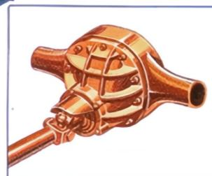
Ford's new exclusive deep-offset hypoid rear axle makes possible its low-to-ground dimensions . . . brings you smoother, quieter operation, longer car life. This axle's new hypoid gears
