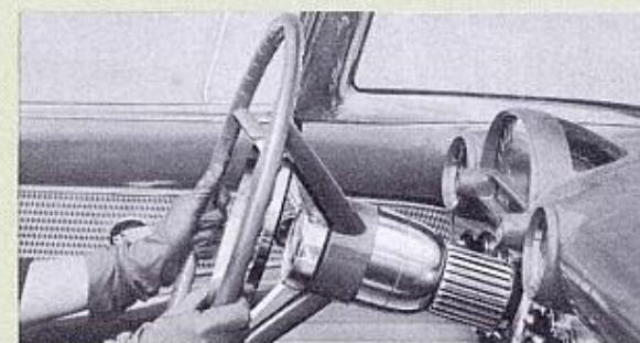
New deep-center Lifeguard steering wheel acts as a cushion to protect the driver's chest from the unyielding steering column, should he be thrown forward in an accident. Wheel position is telescopically adjustable.
