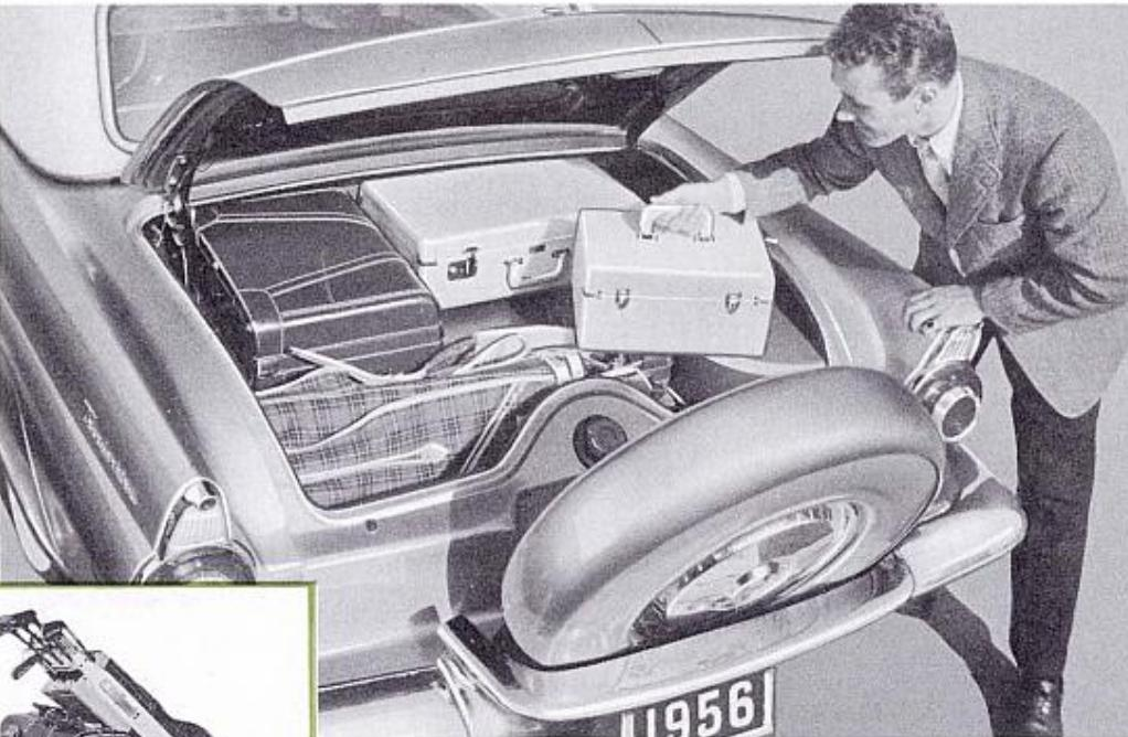
With the spare tire mounted *outside*, there's space for all the luggage you see at left, and more, in the Thunderbird's big new luggage compartment. New spare tire mount moves down out of way on hinged bracket. Deck-lid pops open on counterbalancing hinges when you turn the key.
