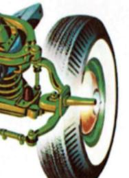
*Ball-Joint Suspension*, with its wide-spread control arms, is retained in all 1956 Ford models. It keeps wheels in line longer and has anti-bind seats for consistently easy handling . . . simplifies servicing.
