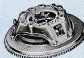
Heavy-duty 11" clutch is semi-centrifugal type. (Standard on "Interceptor" V-8 with Conventional Drive or Overdrive.)
