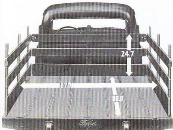
**Strong, spacious platform** is 6½ ft. long, 5½ ft. wide! Stake and rack boards are straight-grained, seasoned wood. Stake racks are held firmly at the top by strong, interlocking steel plates. Stake pockets are flush with floor for unobstructed open platform use. Heavy steel rub rail and steel caps on body ends protect platform.
