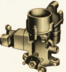
**NEW TYPE, DOWNDRAUGHT CARBURETTOR** (left) and new design of induction exhaust manifold incorporating a fully automatic heat control valve (right) contribute to the engine power-output and flexibility which give Prefect and Anglia their very remarkable top gear performance.
