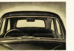
**DUAL SCREEN WIPERS** with an efficient sweeping over a very large area these two vacuum operated wipers keep vision clear in the heaviest weather.
