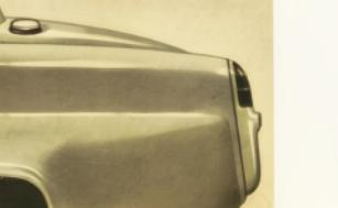
**HIGH POSITION FUELING CAP.** Located high on near side rear quarter panel, petrol tank filler neck allows easier and faster fuelling service.
