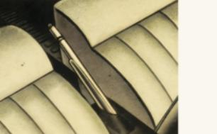
**A PULL-UP TYPE HANDBRAKE.** Immediately at driver's hand between front seats with long, easily released lever for powerful and quick application.
