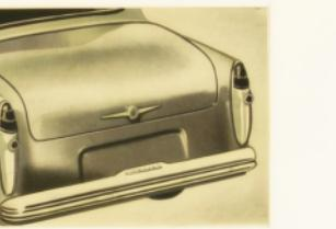
**TWIN TAIL LAMPS.** Assemblies include flashing traffic turn indicators operating in combination with similar flashers in the front parking lamps.
