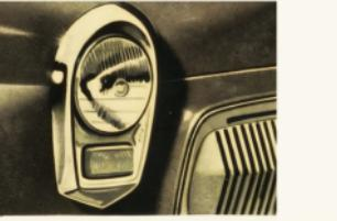
**COMPACT HEADLAMP ASSEMBLY.** Encasing of headlamps and built-in combined parking and traffic flasher lamps is a smart, practical feature.
