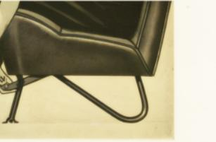
**ADJUSTABLE FRONT SEAT.** At finger tip pressure a spring-loaded lever adjusts Prefect's front seats and Anglia's driving seat over a range of 4 inches.
