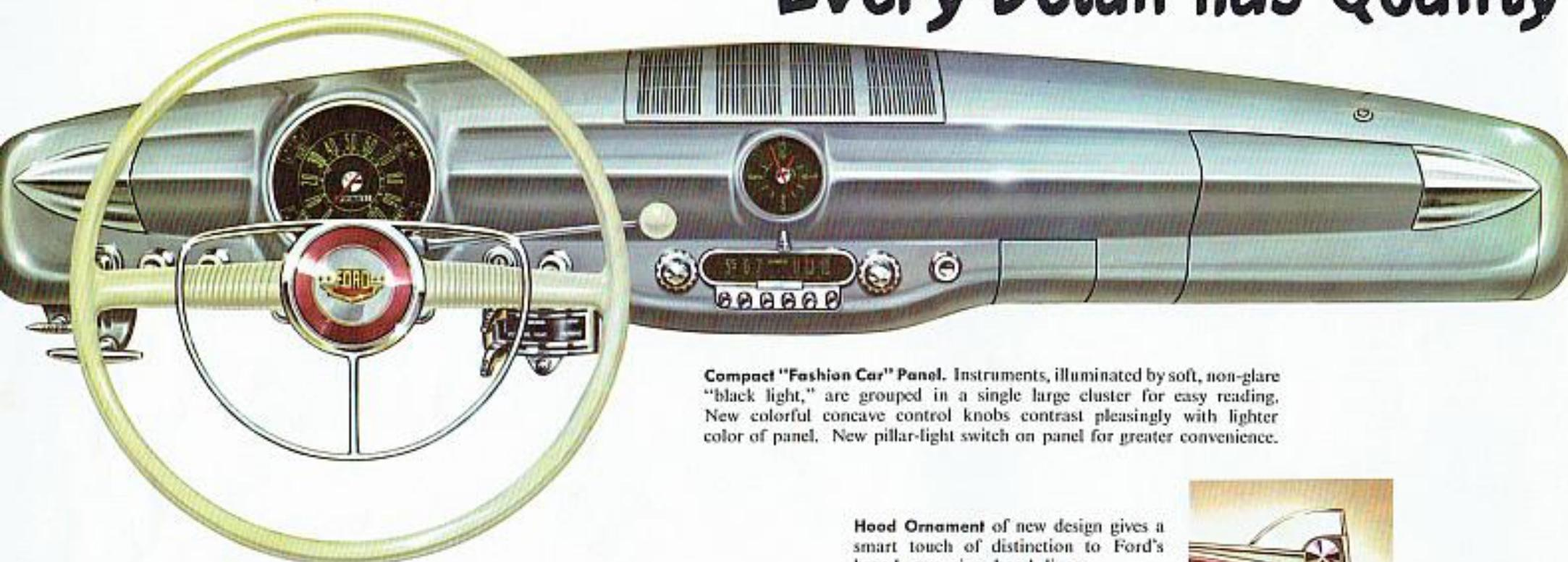
**Compact "Fashion Car" Panel.** Instruments, illuminated by soft, non-glare "black light," are grouped in a single large cluster for easy reading. New colorful concave control knobs contrast pleasingly with lighter color of panel. New pillar-light switch on panel for greater convenience.
