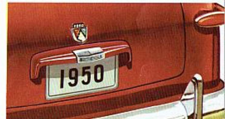
**New Deck-Lid Handle** incorporates new trigger-type latch. Makes attractive frame for license plate. Permits easy access to roomy, weather-sealed luggage compartment.
