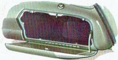
**New Double-walled Glove Compartment Door** has new piano-type hinge. It looks better—and it works better.
