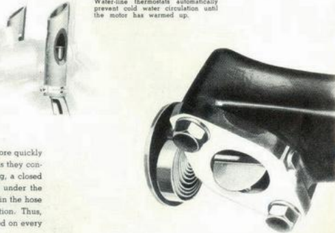
Manifold Heat Control, which is closed when motor is cold, automatically routes hot exhaust gases under carburetor until motor warms up.
