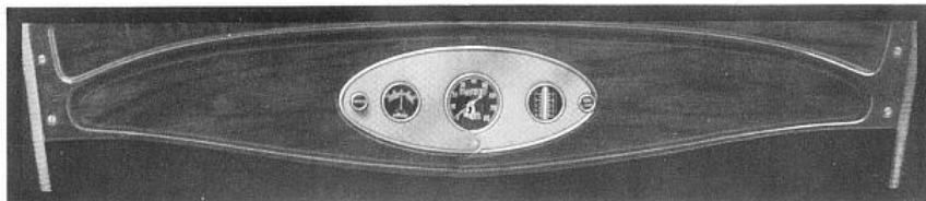
Note how all instruments are grouped within easy reach and view. The panel is indirectly lighted, eliminating all glare.
