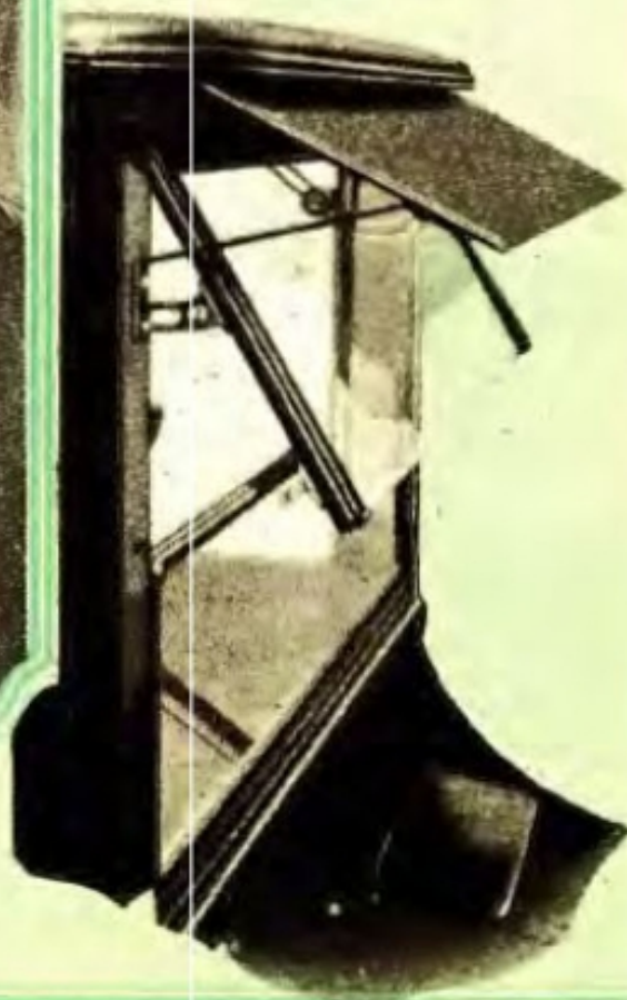
A COWL VENTILATOR, sun visor, and adjustable upper windshield glass are standard equipment on all Ford enclosed body types
