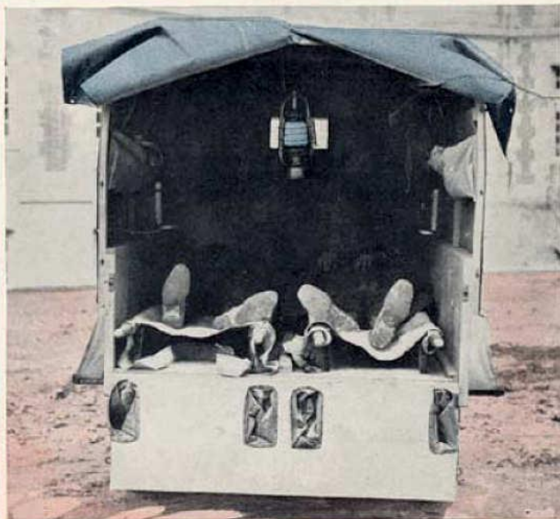
Showing how wounded soldiers are carried on army stretchers. Note pockets in tail board to receive the ends of the stretcher
