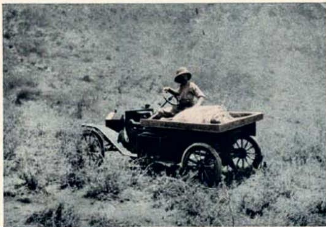
Ford army transport with body made of old packing case, B. E. A.
