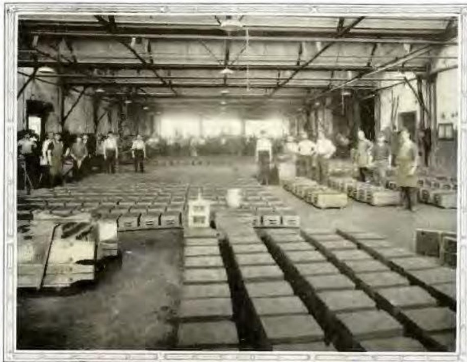
THE GREAT FOUNDRY'S main room. Three hundred cylinder moulds ready for the molten iron. Fans remove all dust and smoke
