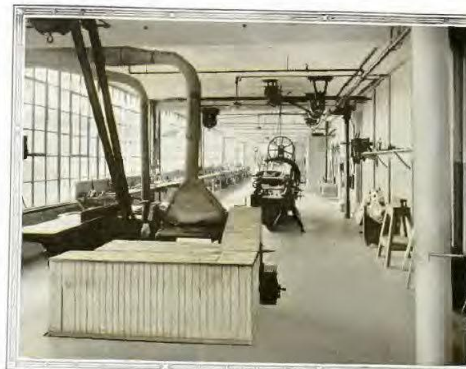
PATTERN SHOP that furnishes the wood patterns from which the foundry makes its castings. Note the individual motors for each machine
