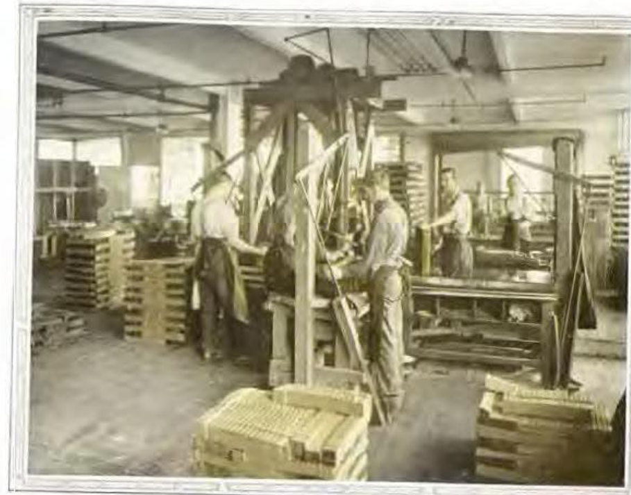
AN INGENUOUS MACHINE in the radiator department. It is typical of Ford methods, doing the work of ten men by the pressure of a lever
