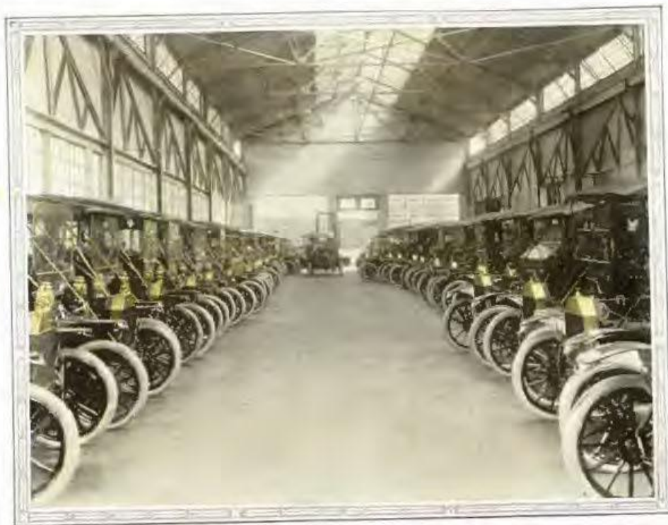
EIGHTY MODEL T's receiving their final test. The rear wheels are jacked up and the engine and all working parts are given a thorough trial
