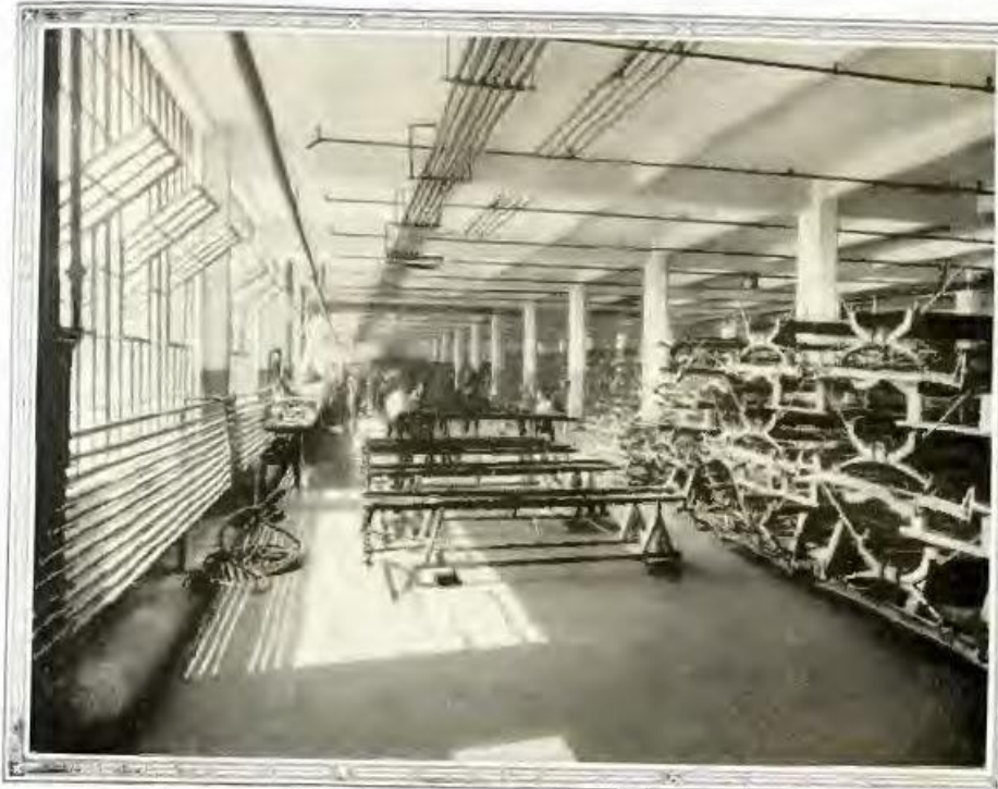
ASSEMBLING ROOM NO. 1 —Here the bare chassis frames receive their preliminary equipment of fender irons, springs, brake levers, etc.
