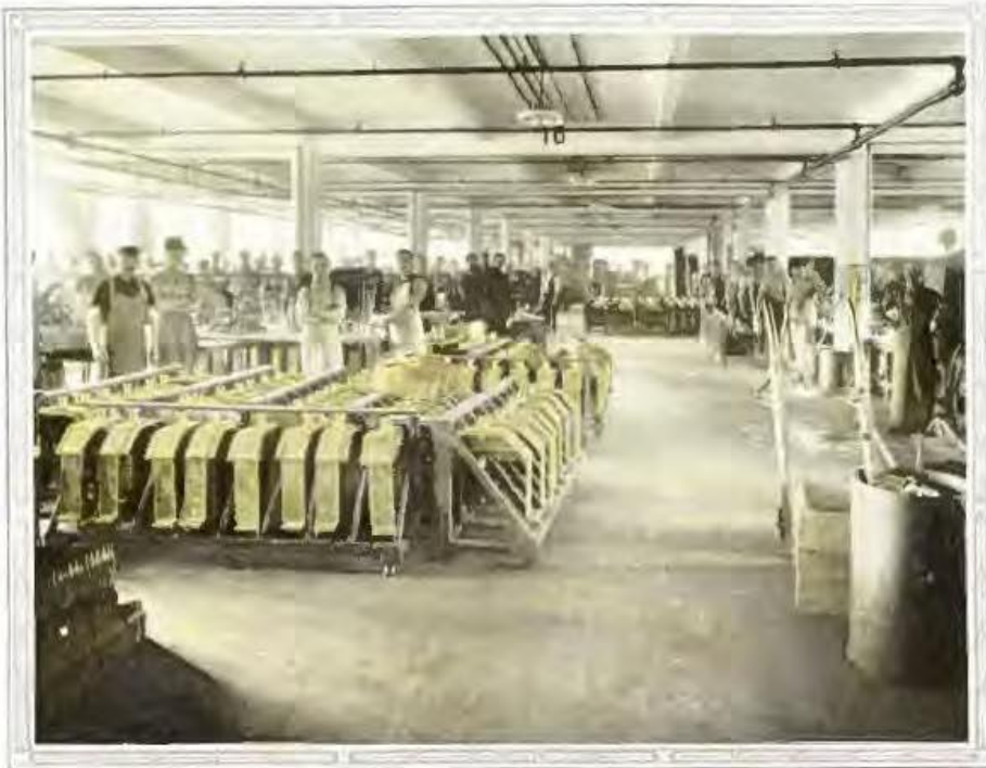
RADIATOR DEPARTMENT —Three hundred men are needed to make Ford radiators as fast as they are required—250 per day
