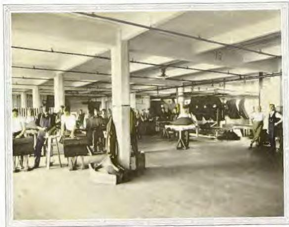
LACQUERING FENDERS, hoods, fuel tanks and other parts. Each is dipped in a big vat, hung up to drip and then baked hard and glossy
