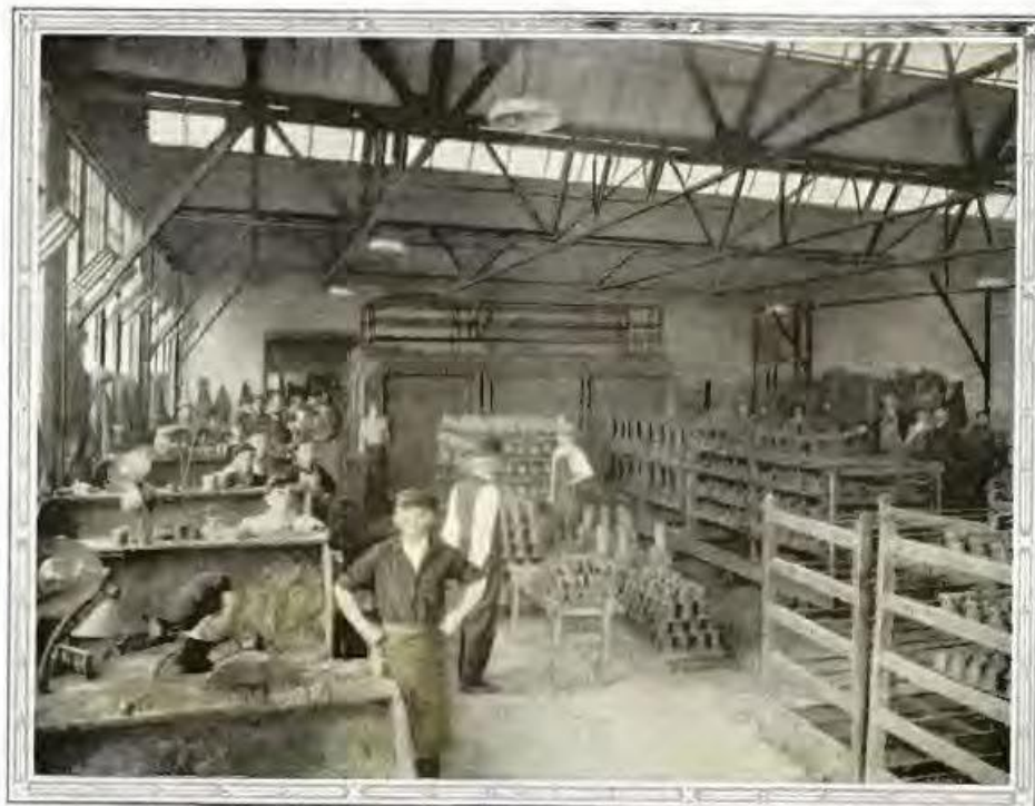
CORE ROOM —The cores are made of adhesive sand, baked hard and are used to form the "holes" in hollow castings
