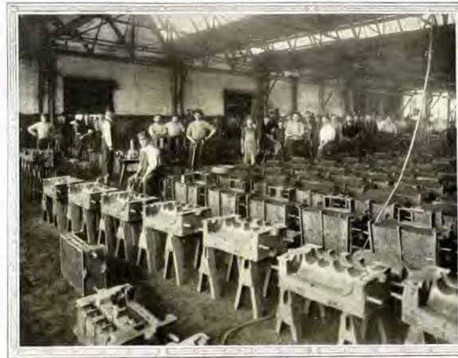
MOULDS receiving the finishing touches. Their interiors are dusted with graphite, insuring smooth, clean surfaces on all Ford castings
