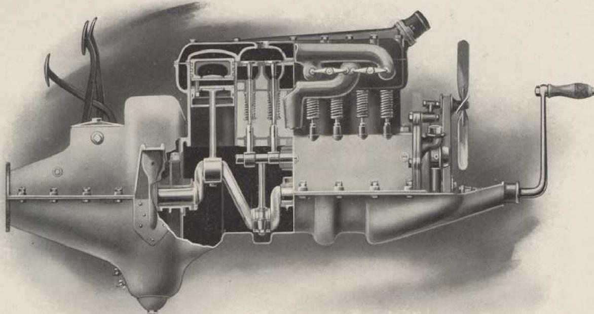
Semi-Sectional View Model T Ford Power Plant
