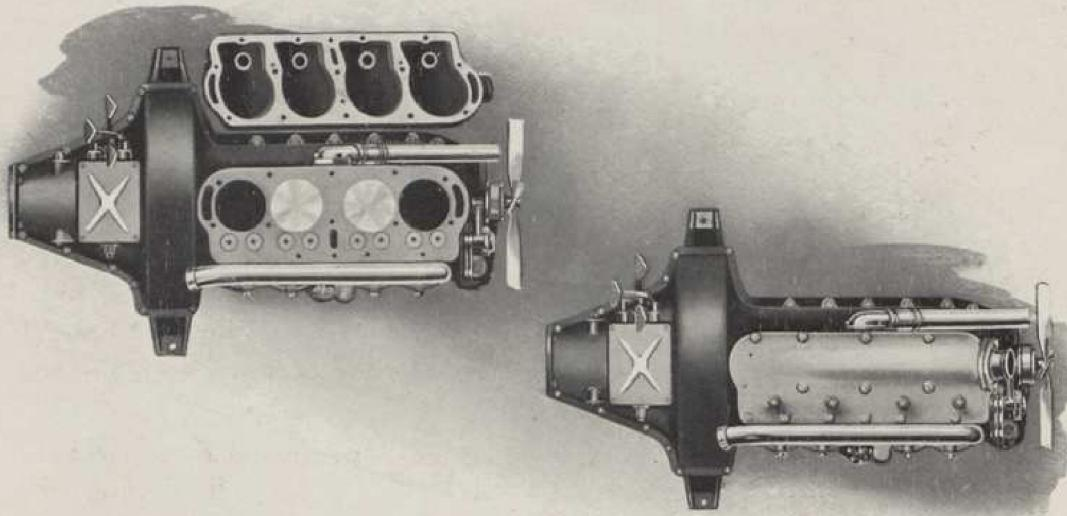
Showing Construction of Cylinders
