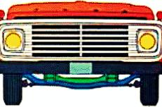
**Wide-track maneuverability** and outstanding vehicle stability are attained with Ford's wide-track front axles that allow wheels to turn up to 44°. This cuts the need for backing on tight turns, promotes greater safety and better schedules.
