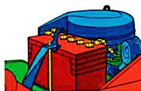
**Engine compartment location of battery** permits more frequent and better servicing. Two batteries, one on each side of engine, are supplied on most Diesel-powered buses. Optional 204 amp-hr battery is frame-mounted and connected with 36-inch slack wire.
