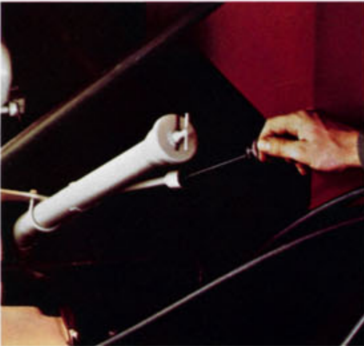
Both oil dipstick and filler pipe extend from the engine to the back of the cab. You can check or add oil with cab in place.
