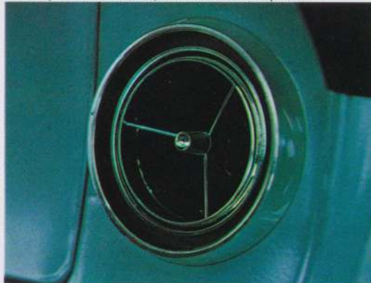
Adjustable air nozzles at either end of instrument panel direct air for maximum air flow.
