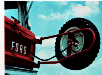
Swing-Away Outside Spare Tire Carrier gets the tire out of the way for easy access to rear cargo area... allows increased cargo or luggage space.
