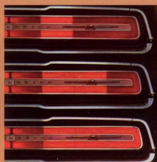
Sequential Turn Signals indicate turn direction in rippling flow of light.
