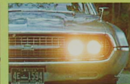
Latticework grille folds back, revealing Thunderbird's headlamps.
