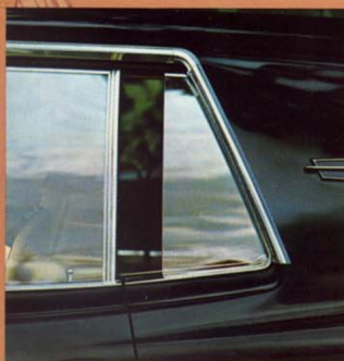
Sliding Quarter Windows on two-door models slide smoothly into roof pillar.
