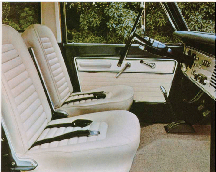
Front Bench Seat. A three-man, full-width front seat is standard on all Broncos and is upholstered in Parchment-colored vinyl trim. Front seat travel adjustment is five full inches.
