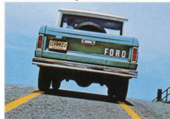
Stability . . . A wide 57.4-in. track for Bronco's front and rear axles reduces side sway on the highway and provides trail-hugging stability when traversing steep hills.
