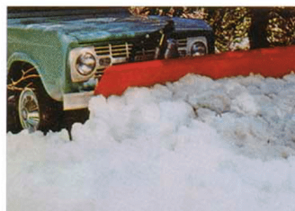
Snowplow . . . If you live in snow country, equip your Bronco with a snowplow. Controlled from the cab, the blade may be adjusted to various heights and angles for most effective use.
