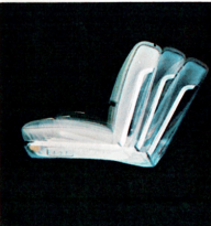
6-WAY POWER SEAT. Front to rear, height and tilting adjustment provide quick, effortless regulation to your favorite driving or sitting position. Full-width seats and driver's seat in XL and 7-Litre models. (Not available in full-width seat with 4-speed transmission.)
