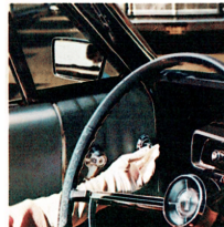
VISIBILITY GROUP. A three in one group including: remote control outside mirror (which is easily adjustable from inside the car), day/night inside mirror (dims annoying nighttime headlight glare) and 2-speed electric wipers.
