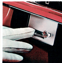
AUTOMATIC SPEED CONTROL. Ideal for turnpike cruising. Set dial (25-90 mph) and accelerate to selected speed. Take your foot off the gas pedal and speed control does the rest. Maintains selected speed even up and down hills. Disengages at a touch of the brake.
