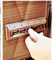
POWER WINDOWS. Control all four windows from the driver's seat as easily as pointing your finger. Individual passenger controls. Driver's master control panel has fifth button to "lock out" all but his own if desired.
