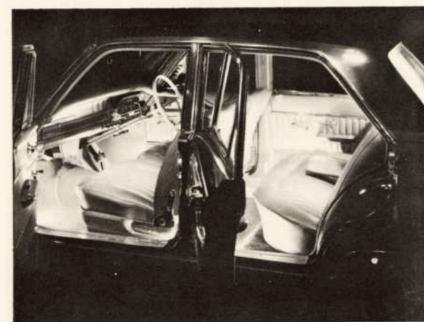
Fairmont introduces a new elegance in lighting. The entire floor is flood-lit as you open any door. (The lights are concealed under the fascia panel, and at the base of each of the centre pillars.)
