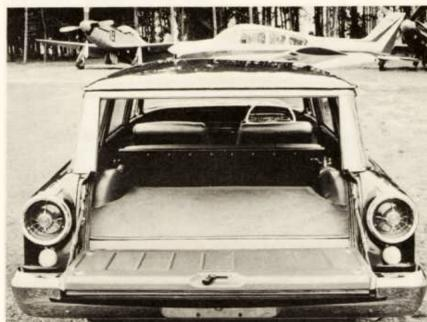
Deep, cut-pile carpeting extends right through to the tailgate. Two roof lights are provided — a centre dome light operated by the headlight switch rheostat; another for lighting the rear load area is located close to the tailgate window and is operated by its own individual switch.
