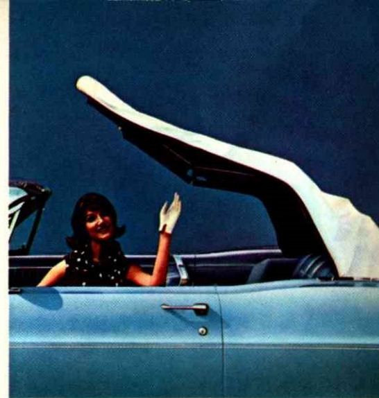
New convertible top is constructed of rugged 5-ply satin finish vinyl for durability. Glass rear window (standard) resists scratching, discolouring and can't wrinkle. Power top (shown above) is optional.
