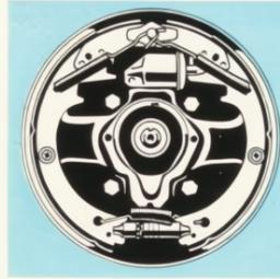
The heavy-duty hydraulic brakes, have had their total lining area increased to 238.04 inches. Internal shoe parking brake gives positive holding on steep inclines, supplements 4-wheel brakes in an emergency. You get the maximum stopping power on the move and the maximum security when standing stationary.
