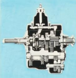
The "New Process 435" 4-speed synchromesh transmission makes best use of F 250's power. New blocker-type synchronizers, integral with the mainshaft, give greater durability, and smooth, quiet gear engagement with little effort by the driver. It provides more pulling ability and economical operation than 3-speed transmissions.
