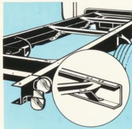
Ladder-type frame with five cross members has alligator-jaw attachment to side rails. Heavy-gauge steel construction gives great frame rigidity. Frames are of S.A.E. standard "X" width to facilitate mounting of standard or custom-built bodies. It gives you a lot of extra strength, durability and payload capacity where it counts.
