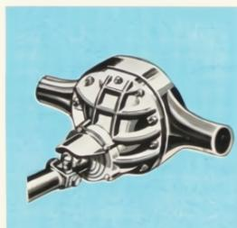
The rugged full-floating hypoid rear axle has a rated capacity of 7,400 lbs. Heat-hardened alloy steel construction prepares it to take shocks and strains, and more accurate ring gear alignment keeps it working for long periods without adjustment. All gears of alloy steel, heat treated for dependable strength and durability.
