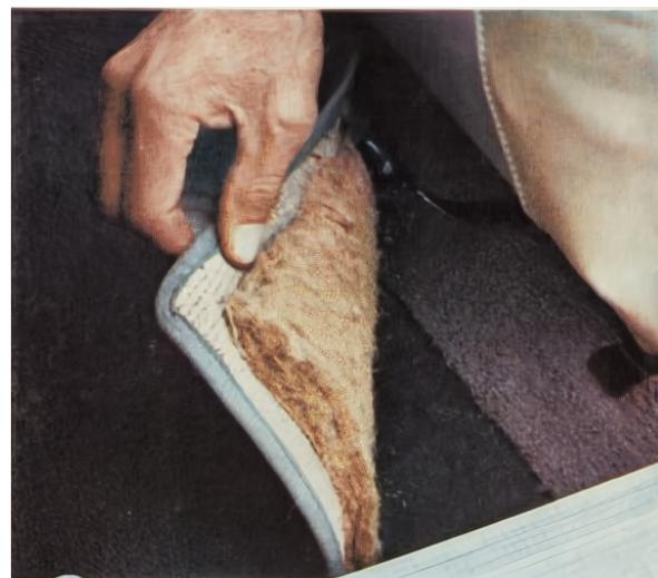
Insulating and sound-proofing materials completely surround the passenger compartment to absorb noise *before* it enters the interior. The engine hood, interior floor, and roof are lined. Undercoating, too, deadens road noise as well as protects Falcon's underbody against rust and corrosion.
