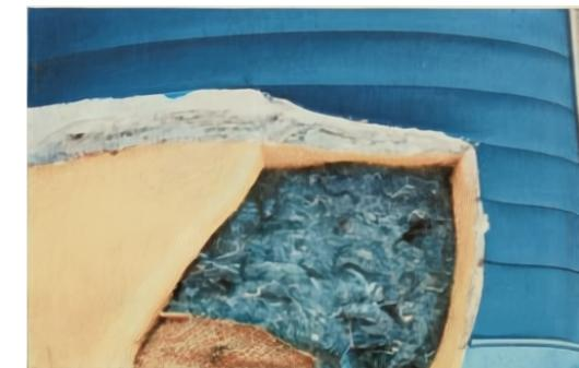
All Falcon's seats provide the deep-down comfort of foam and wool cushioning. New springing provides firm support, prevents seat "sag", and lasts longer. New "Glove Grain" vinyls, too, are more durable, wipe clean with a damp cloth.
