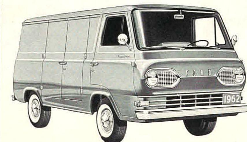
**Econoline Van** has a big 204 cu. ft. of loadspace with full height wide side and rear loading doors. Built right through for top economy, it hauls payloads up to 1650 lbs., has a tight 34.5 ft. turning circle. Choice of economical 85-hp or 101-hp six cylinder engines.
