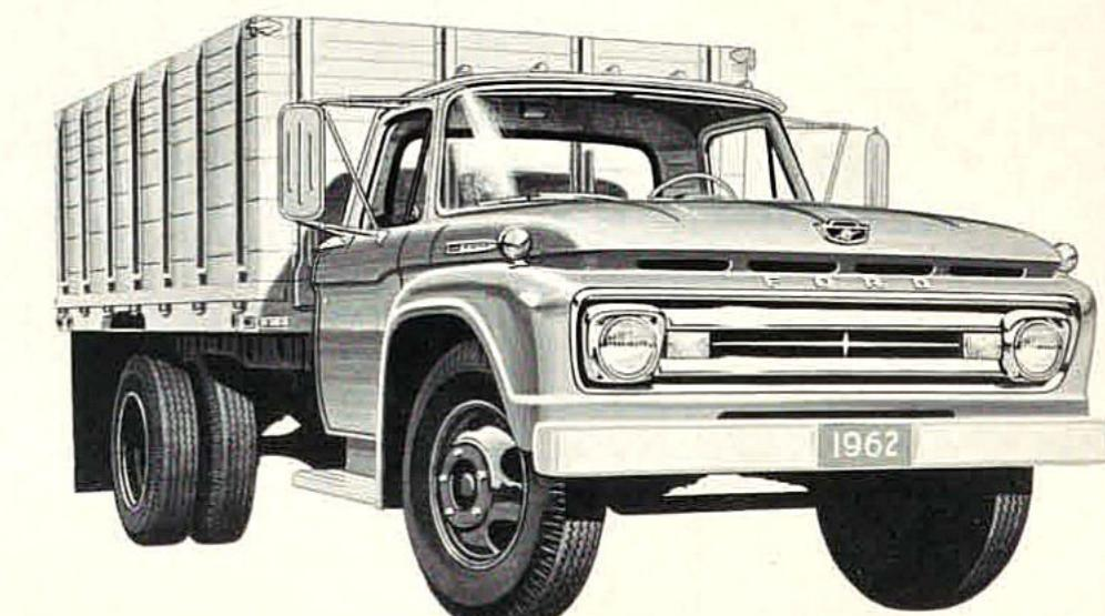
**F&M-500's** have a wide choice of economical power —Six or V-8. The 135-hp six, low-priced 160-hp V-8 or the 171-hp HD V-8 are all available for top performance on any job. Wheelbases up to 174 in. accommodate bodies up to 15'; GVW to 15,000 lbs.
