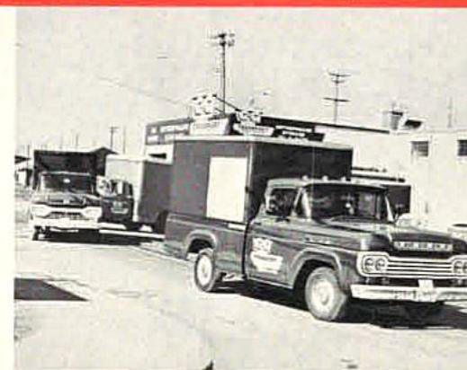
**GG TRANSPORT** owns two of these new 1961 C-700 Tilt cabs. This one has a 175" wheelbase with a 22 ft. van. It has the 302 engine, 5 speed transmission with 2 speed rear axle, wide track front axle. They have 23 Fords in their fleet now and are replacing all units with Fords.
