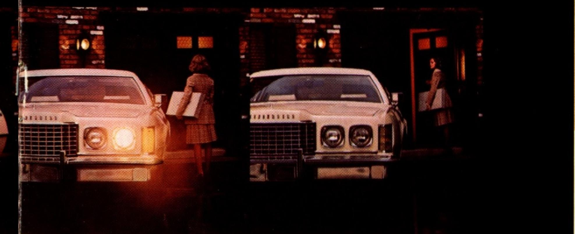
**New Autolamp On/Off Delay System.** Included with the Light Group detailed above, automatically turns driving lights on or off in response to light conditions. The Autolamp System also lets you leave headlamps on for up to 90 seconds so they will help light your path away from the car. Delay period can be adjusted for 30, 60 or 90 seconds. Headlamps turn off automatically.
