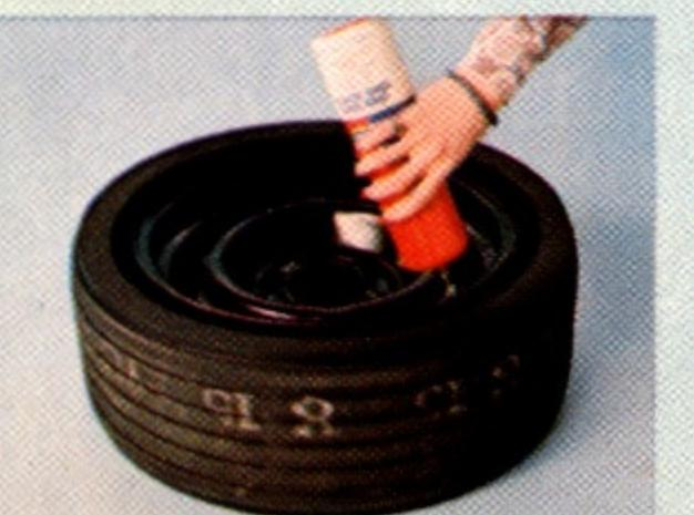
**Space Saver Spare Tire.** Makes more luggage compartment room available. Includes collapsible spare tire, wheel, and pressurized inflating cannister.
