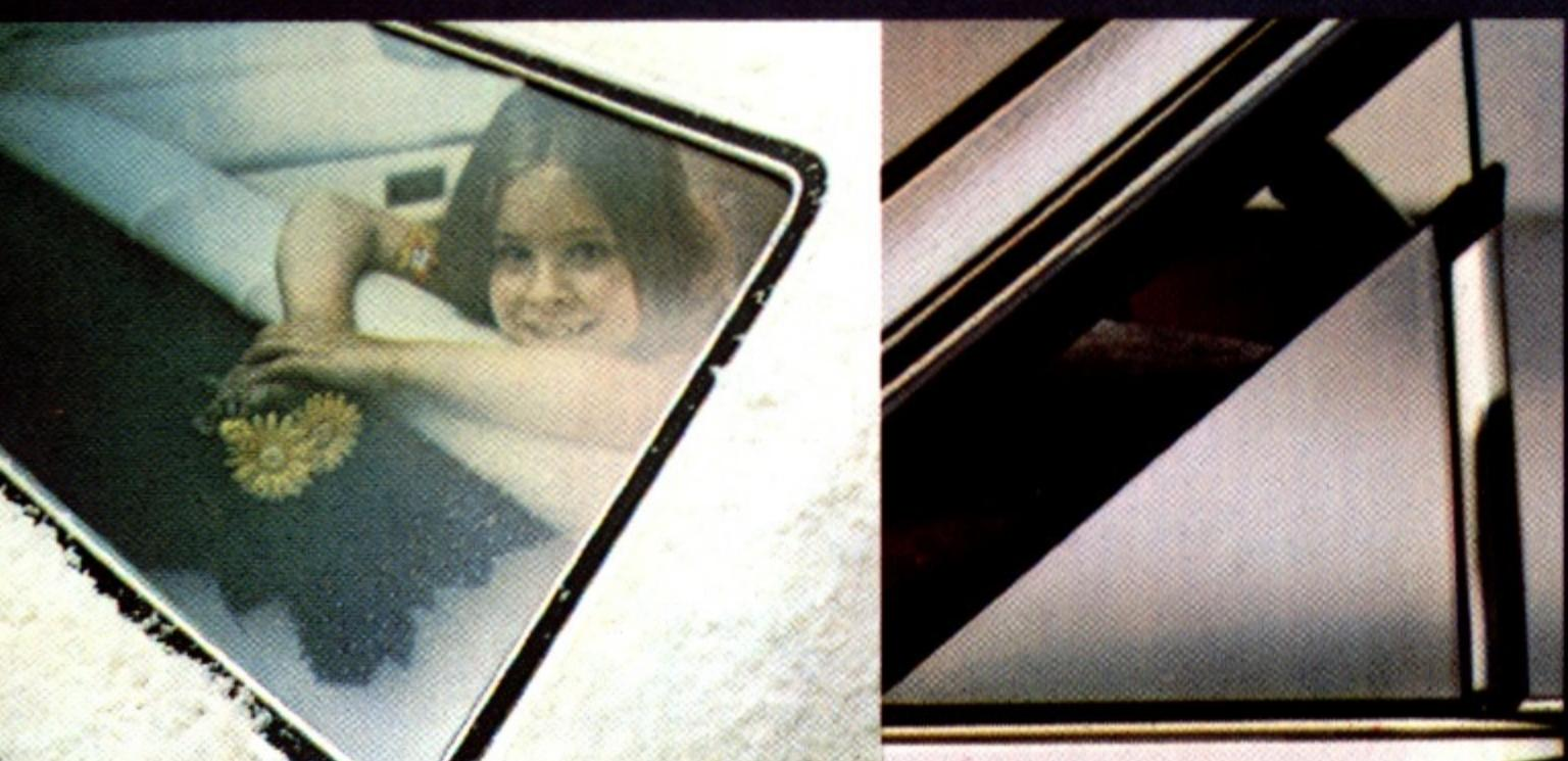
**Quick Defrost Windshield / Rear Window.** New Gold film, laminated in glass, quickly helps melt snow and ice. **Electric Rear Window De-icer** uses fine heating elements to help clear rear window.
