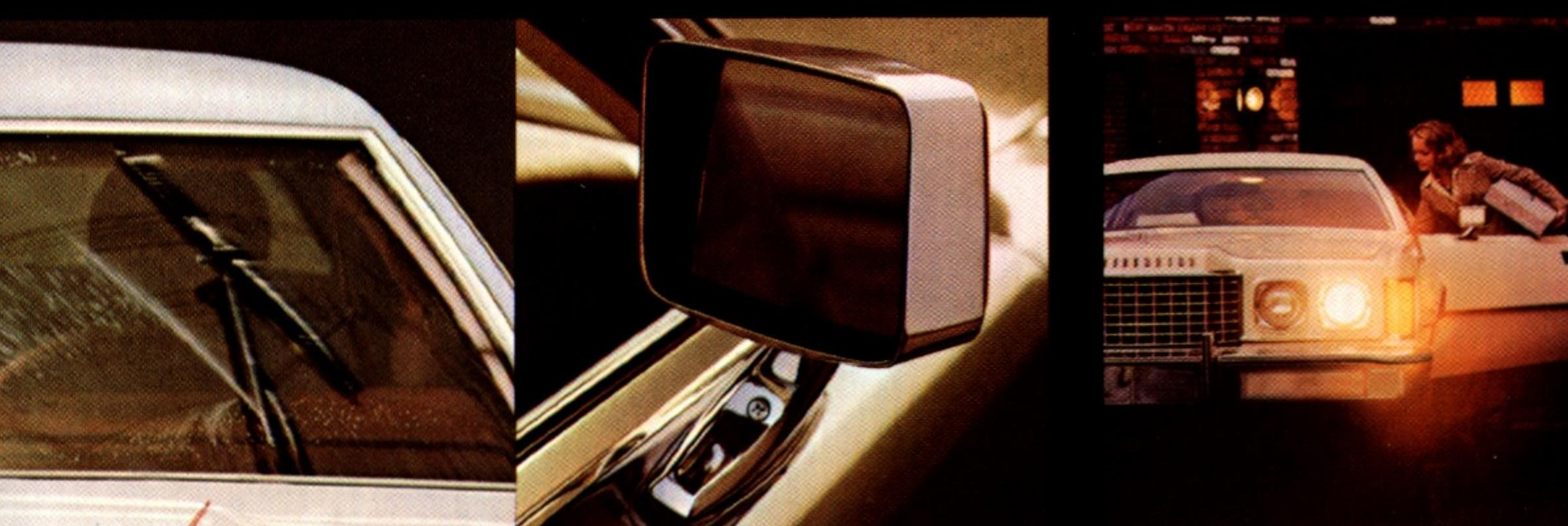
**Convenience Group.** Two handy items. Remote control right-hand mirror, adjustable from driver's seat. And interval windshield wipers which let you regulate pause between sweeps from 2 to 10 seconds to handle road splatter, light rainfall, for best visibility.
