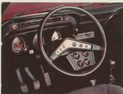
Full Cortina GT instrumentation including: 0-130 mph speedometer, tachometer, oil pressure, water temperature, alternator, fuel gauge, and electric clock.
