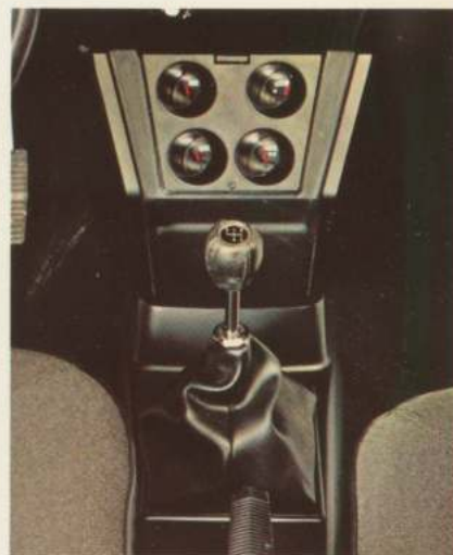
4 speed close-ratio manual transmission with leather covered shift knob.
