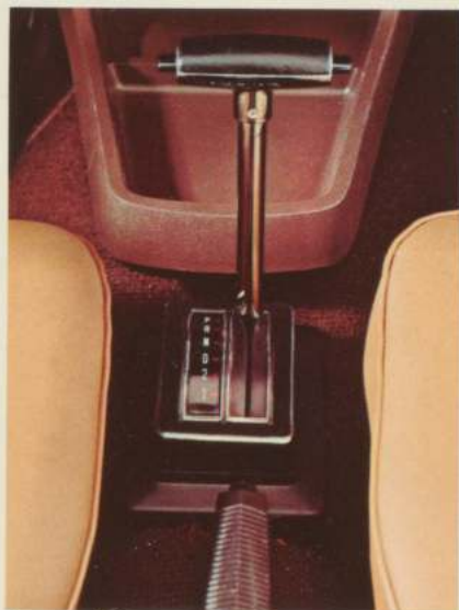
3 speed floor-mounted automatic transmission with console.
