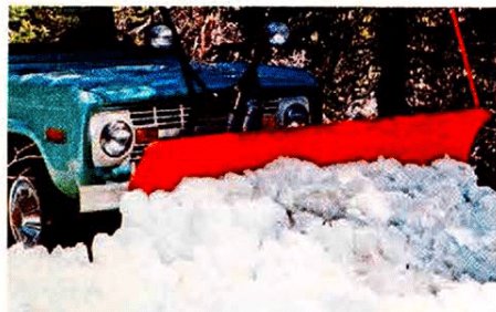
Snowplow Blade may be adjusted easily to various heights and angles (with kit) from within the cab.
