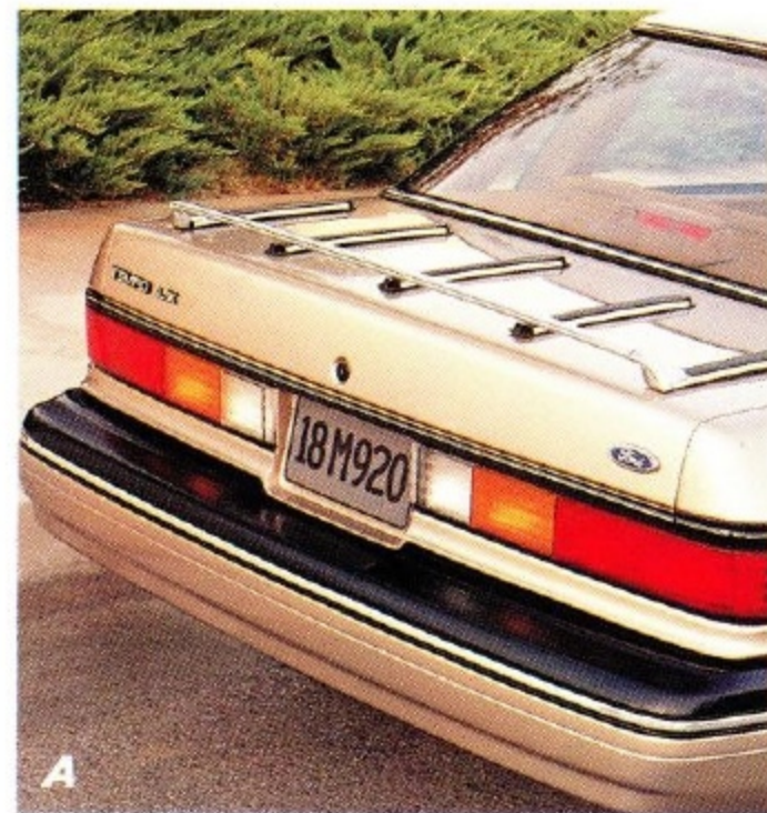
(A) Decklid luggage rack, available on GL, LX, GLS 4-door and AWD models.
