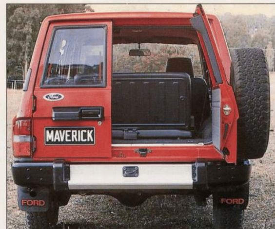
60/40 rear door and third row fold-down rear seat – XL Wagon.
