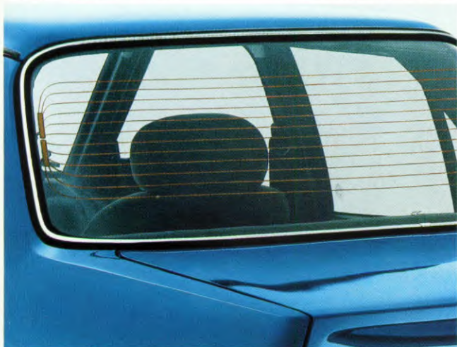
Radio-antenne in verwarmingselement (i.c.m. getint glas).
