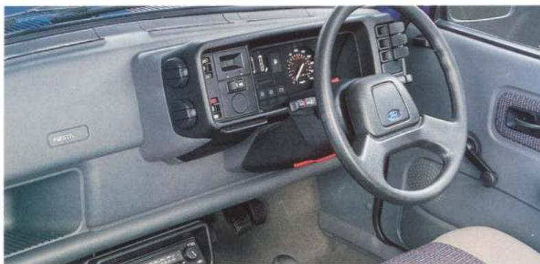
■ Instrument panel features include a 'lights on' warning that avoids the risk of returning to a flat battery. Switches are easy to see, identify and operate.
