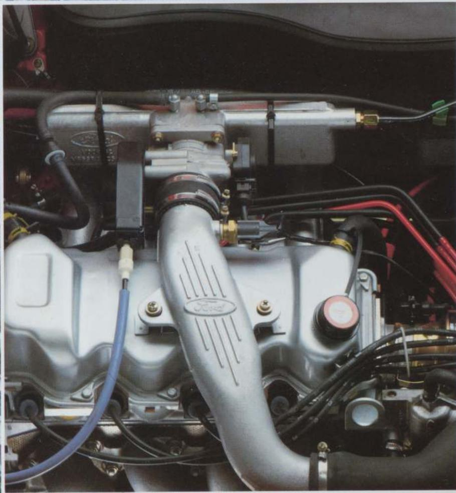
The 1.6i CVH engine fitted to the Escort RS Turbo works in conjunction with a Garrett T3 turbocharger, Bosch KE-Jetronic fuel injection and an air-to-air intercooler to produce an adrenalin pumping 132 PS at 5760 rpm.
