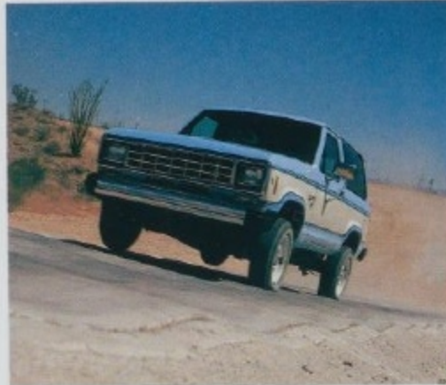
Power Hop Hill tests the ability of Bronco II's drive train components to withstand severe shock loading at Ford's Arizona Proving Ground.
