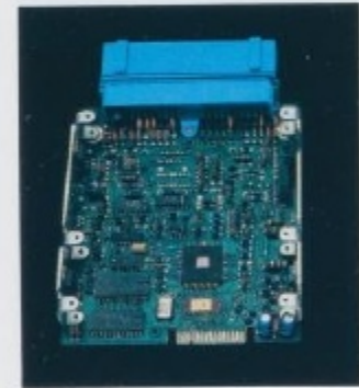
Bronco II's EEC-IV electronic engine control system
