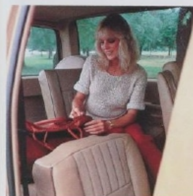
Split fold-down rear bench seat. Fold both seats forward for cargo; one seat forward for cargo and a passenger.
