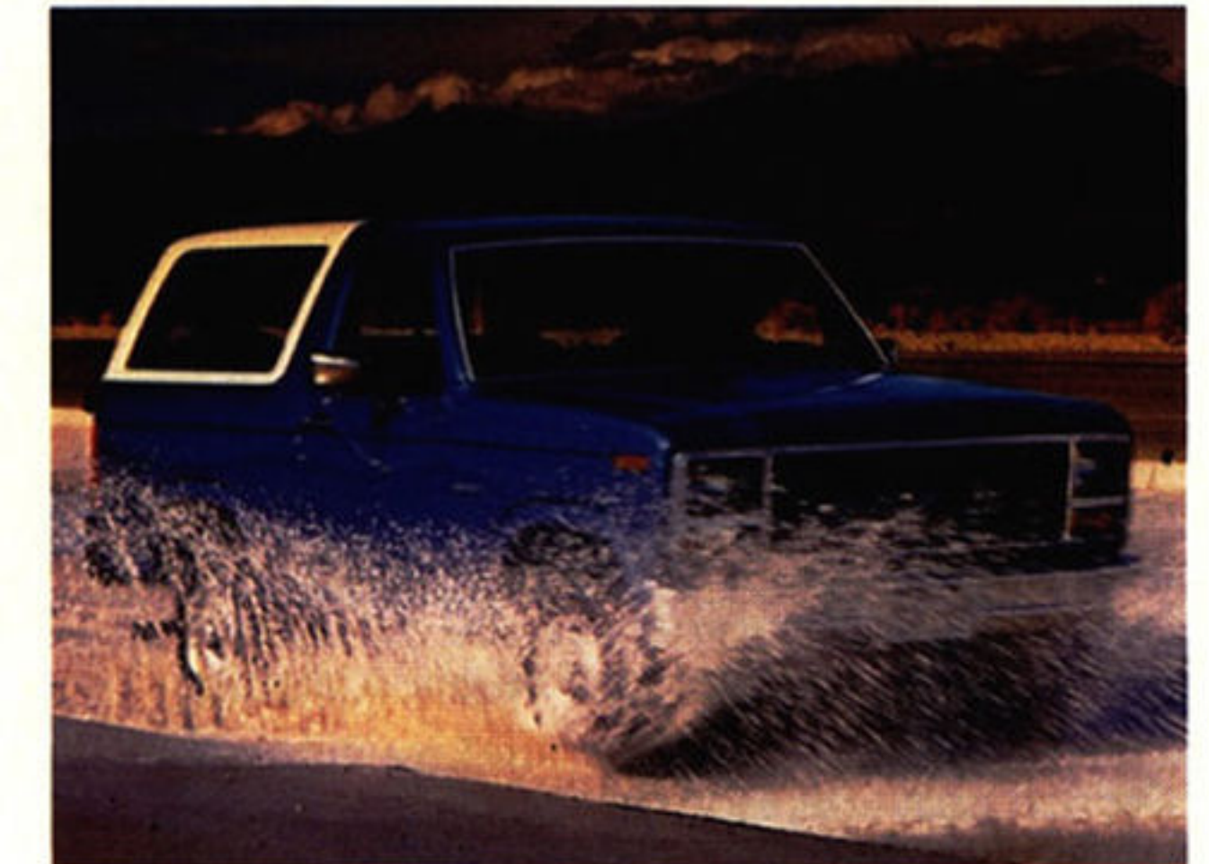
At Ford's Arizona Proving Grounds, extensive corrosion testing includes a salt bath, which exposes all areas of Bronco's underbody and engine compartment to a corrosive spray.
