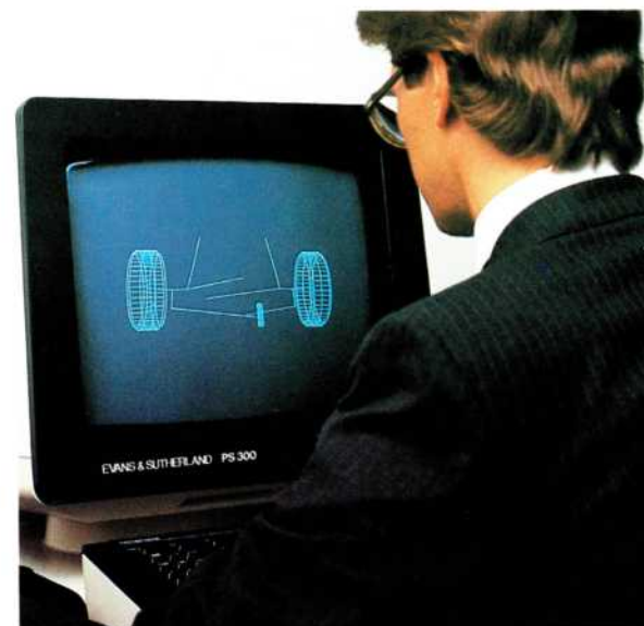
Components of Ranger's Twin-I-Beam front suspension were computer-tested through simulation.
