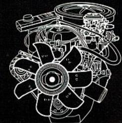
characteristics resulting in a significant lift in power output compared with the previous Alloy Head engine. Driveability during warm-up has also been markedly improved through the fitting of an electrically modulated automatic choke.
