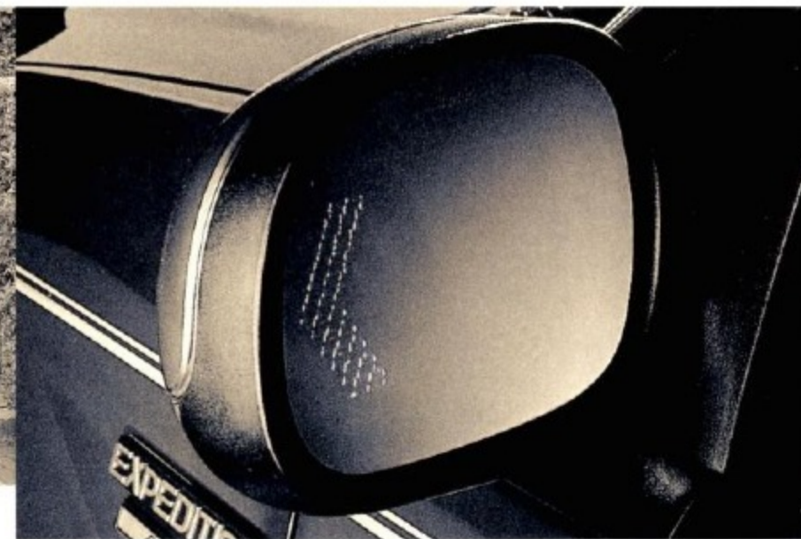
Signal mirrors (standard on Eddie Bauer) display directional arrows invisible to the driver for improved safety while turning or changing lanes.
