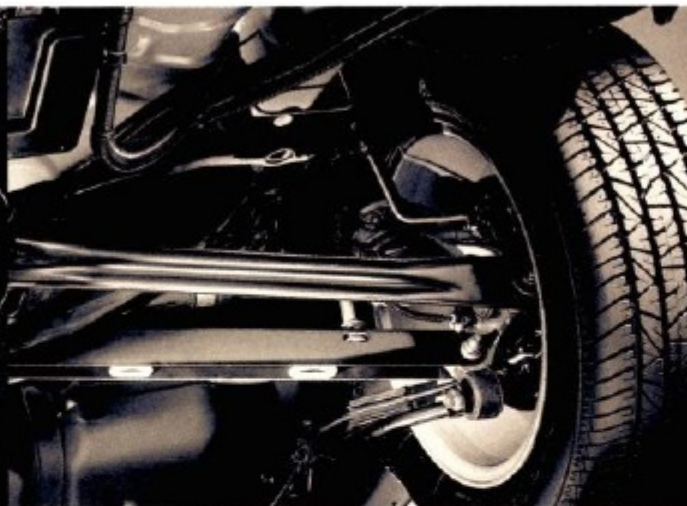
The quadralink suspension system is designed for a smooth ride by keeping all tires level to the ground despite road obstacles.
