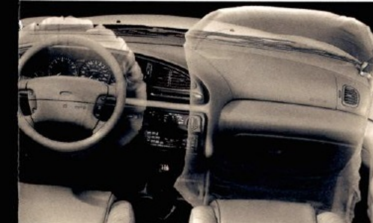
Standard Second Generation dual airbags are depowered to further enhance protection for the driver and passenger.
