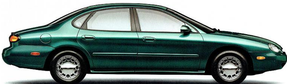
Overall Length 197.5" (sedan) 199.6" (wagon) Wheelbase 108.5" A longer wheelbase allows more space for the passengers inside.
